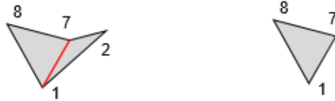
Figure 8. The right polygon shows the ear \langle 1, 2, 7 \rangle clipped from the left polygon.
