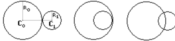
Figure 2. Relationship of two circles, where \mathbf{U} = \mathbf{C}_1 - \mathbf{C}_0 . Left: |\mathbf{U}| = |R_0 + R_1| . Middle: |\mathbf{U}| = |R_0 - R_1| . Right: |R_0 - R_1| < |\mathbf{U}| < |R_0 + R_1| .
